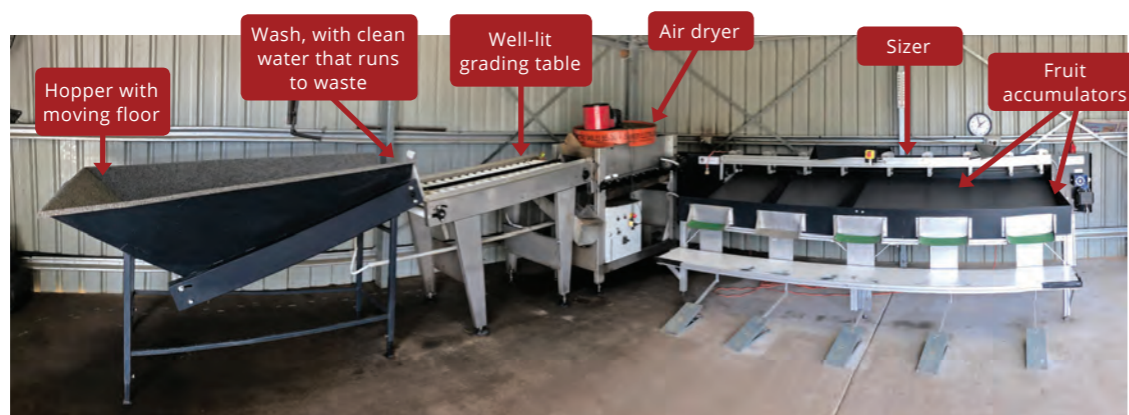
Components of a small but well-designed packing line
