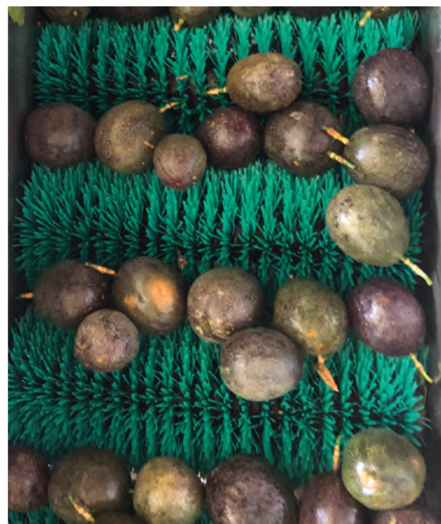
Waxing fruit requires a spray applicator as well as a series of brushes to disperse and polish the coating
