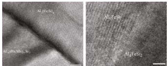
FIGURE 2. High resolution TEM images showing the direct evidence of phase transformation between (a) \text{Al}_{13}(\text{FeSi})_4 / \alpha\text{-Al}_{15}\text{Fe}_3\text{Si}_2 (b) \text{Al}_5\text{FeSi} / \delta\text{-Al}_4\text{FeSi}_2 .
