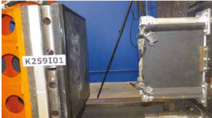
FIGURE 1. Baseline frames (carbon fibre iPanel® + Constellium HSA6™ extrusions) produced in 2017 for dynamic crash testing.
