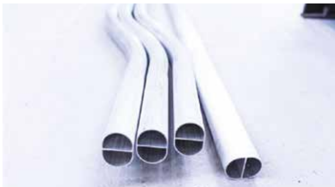
FIGURE 3. CAAHS 3D extruded tubes bent in 2017.
