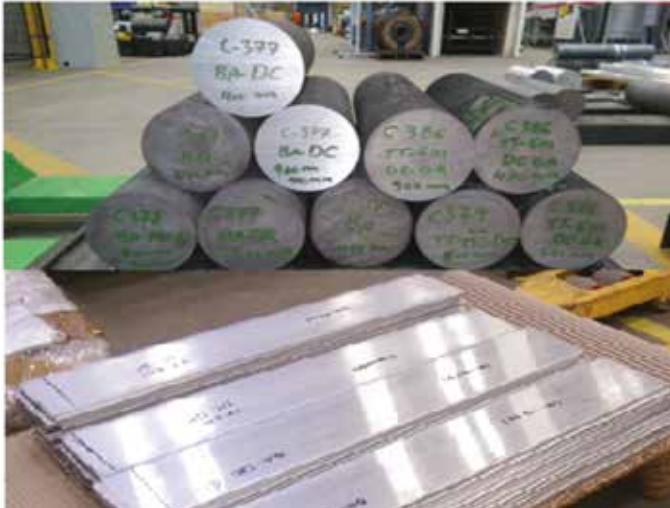
FIGURE 1. DC-GR and MC-DC billets with extruded flat bars of BA-6111 and TT-6111.
