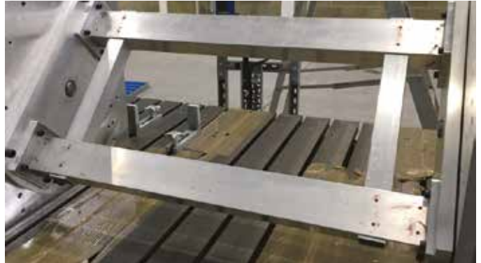
FIGURE 2. Baseline frames produced in 2017 for testing adhesive bonding.
