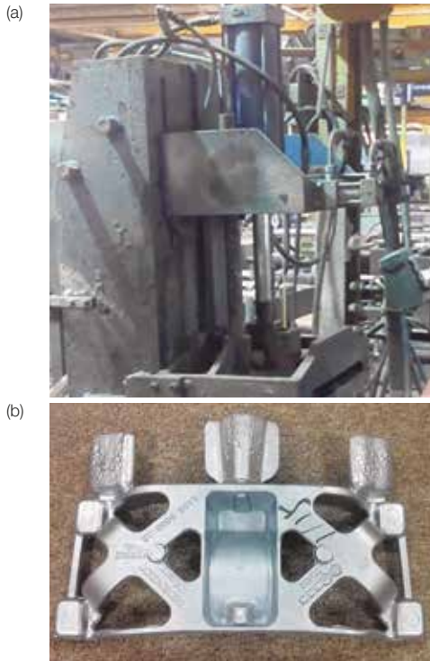
FIGURE 1. (a) Industrial tilting gravity casting trial and (b) trial gravity casting component of the developed aluminium alloy.
