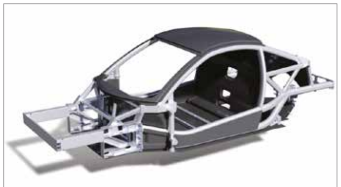
FIGURE 4. CAAHS automotive frame that will be manufactured at scale 1:1 in 2018.
