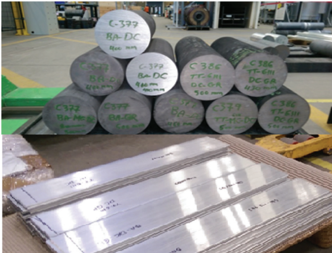
FIGURE 1. DC-GR and MC-DC billets with extruded flat bars of BA-6111 and TT-6111.
