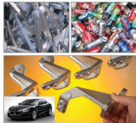
8. Recovery and recycling of secondary aluminium scrap by HSMC with greater tolerance to impurity elements.
