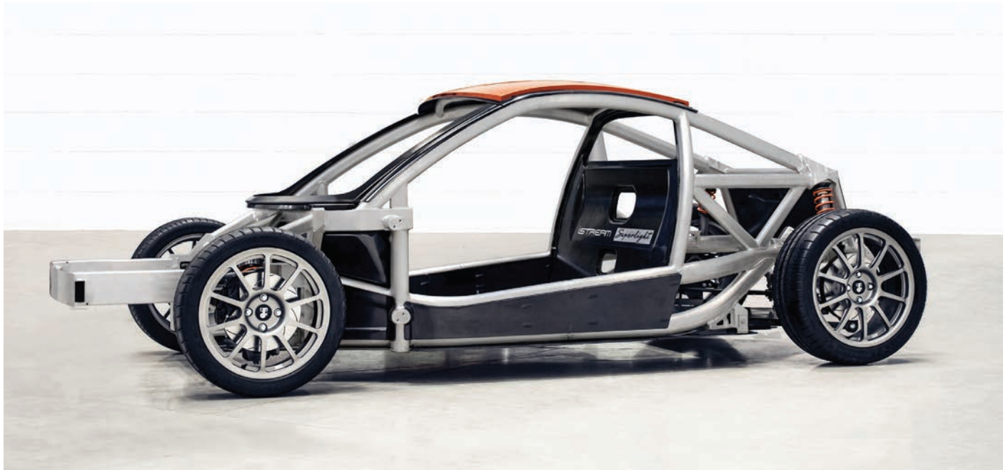
9. Carbon aluminium automotive hybrid structures (CAAHS) structure developed using BCAST's casting and processing facilities.
