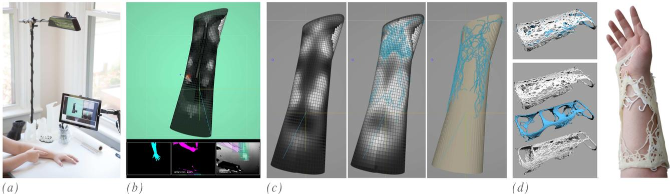
**Figure 1.** Our fabrication-aware design system captures a user’s skin-centric gestures for 3D modeling directly on the body. (a) the system captures skin input on a user’s forearm and (b) translates it to a digital 3D modeling environment model. (c) skin-centric gestures enable the user to create a 3D printable design, (d) which inherently fits the complex geometry of their forearm.
