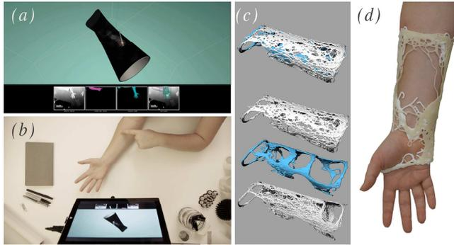
**Figure 11.** An arm brace designed using the generative manipulation mode. (a) skin input updates a touch heatmap of the user's forearm; (b) a design is generated using virtual agents; (c) resulting geometry is processed for fabrication; (d) the resulting physical artifact on the user.
