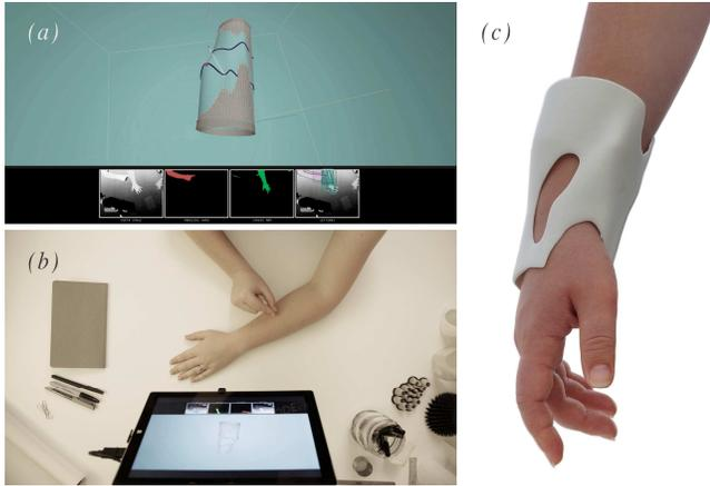
**Figure 9.** An armband is designed using the parametric manipulation mode. (a) skin input updates the arm's base geometry, and simulated rubber bands can be pulled and deformed by the user; (b) the model can be customized to the user; (c) the resulting physical artifact on the user.
