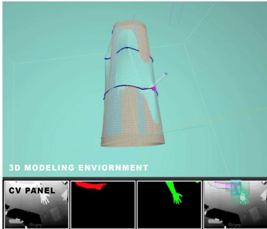
Figure 5. Real-time visual output shows the 3D modeling environment, and a computer vision panel with the raw depth image, modeling hand segmentation, canvas arm segmentation, and hand and gesture tracking.
