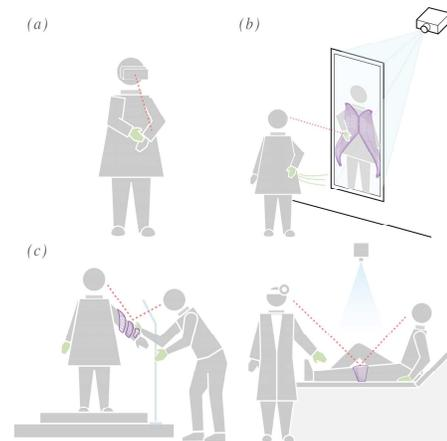
**Figure 2.** The point-of-view of the user or users determine the physical configuration of a skin-centric design tool. (a) first-person systems have a direct line of sight to the user's canvas area, (b) second-person systems have partially occluded canvas areas, and (c) third-person systems enable multiple users to participate in design.
