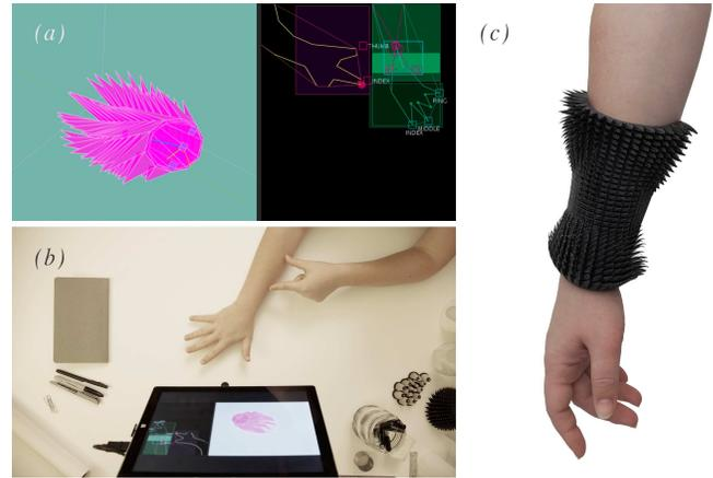
**Figure 10.** A piece of jewelry is designed using the parametric manipulation mode. (a) skin-centric gestures manipulate a pre-designed 3D model, and the animated digital geometry responds to the user's movements; (b) the model is customized by the user; (c) the resulting physical artifact on the user.
