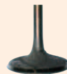
Fuel inlet valve using regular unleaded 91 after 3200km*
