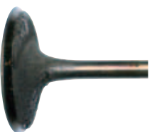
Fuel inlet valve using ordinary fuel* after 3200km
