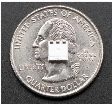
A single NeoPixel device is absolutely tiny, as you can see. They can be used in a daisy chain arrangement, with the output of one linked to the input of the next. A single Arduino pin can be used to control a very large number of lights in this way. Software in the Arduino waggles the data line up and down to signal the amount of red, green and blue the led is to display. When one led has acquired its settings it then passes the signal onto the next one in the chain, and so on.
