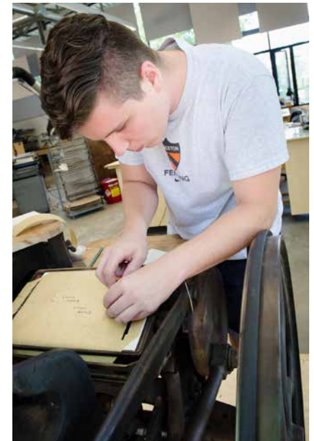
Setting up a clamshell letterpress.
