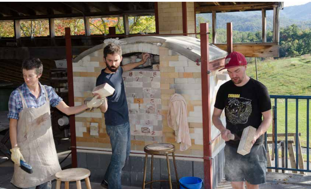
Bricking up the door of the small salt kiln on a beautiful day.
