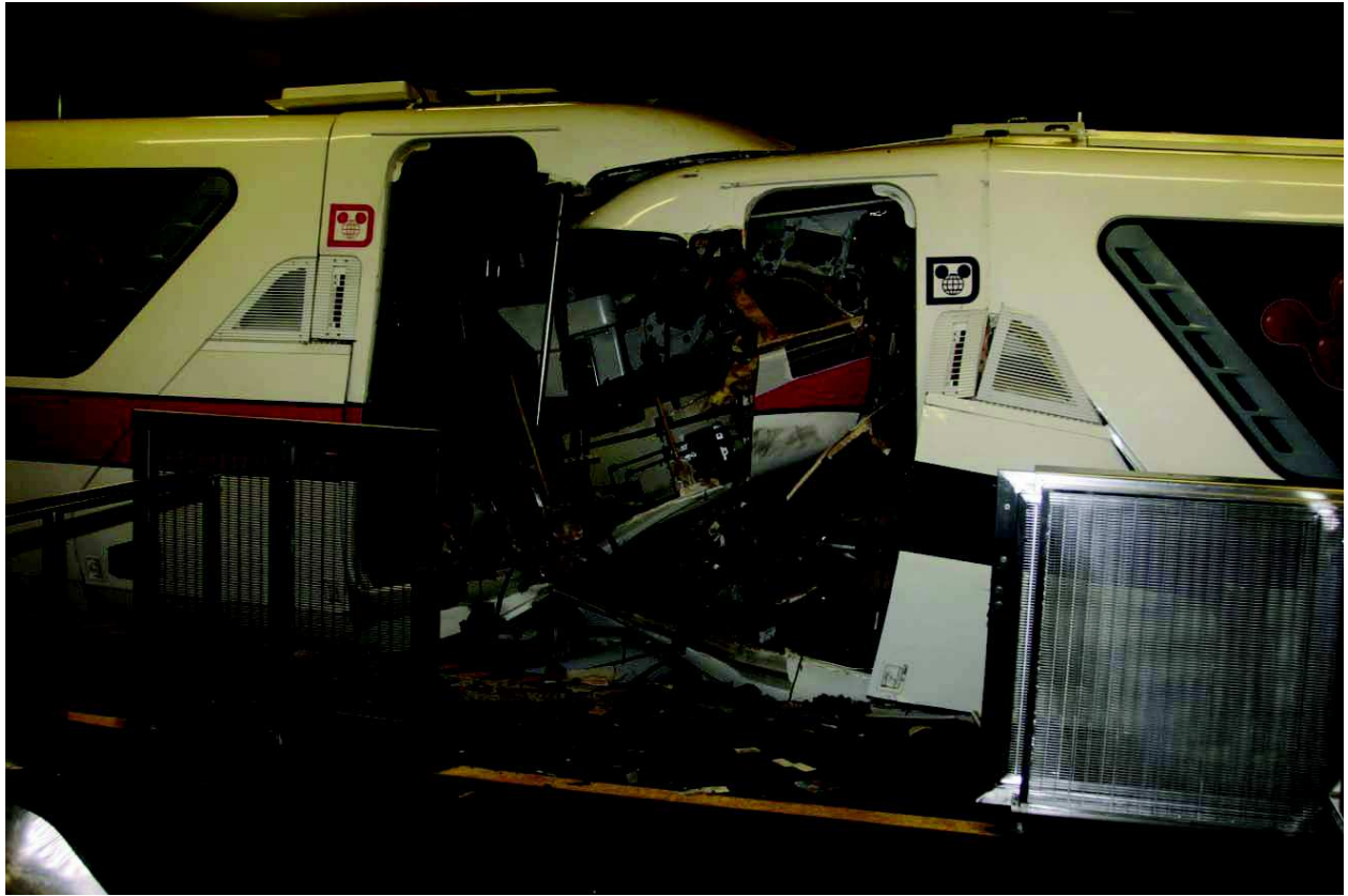
Figure 1. The accident monorails after the collision. The rear operating cab of the Pink monorail (unoccupied at the time of the accident) is on the left, and the front operating cab of the Purple monorail is on the right.
