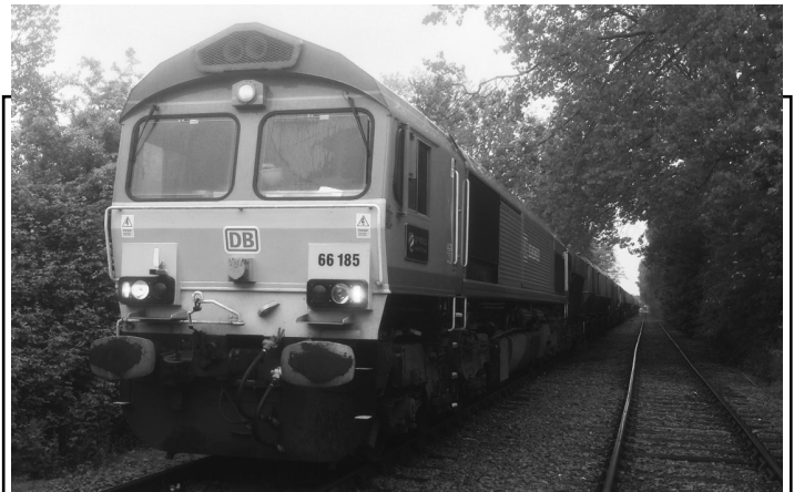
American built Class 66 locomotive #66185 on a train at Elstow Sidings (Bedfordshire) waiting to back out onto the mainline with 42 empty wagons after delivering 1500 tonnes of road stone.
