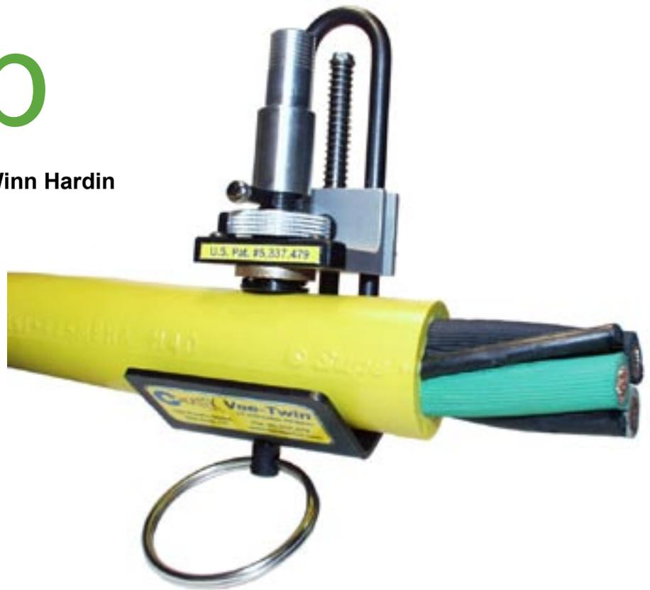
precision vice and moveable razor. The spring-loaded blade retracts into the central housing and a tunable silver dial moves the razor up or down in 0.0 10- or 0.025-inch increments.
