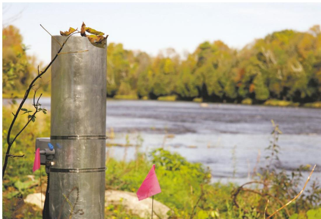
As part of the Beacon Institute's River and Estuary Observatory Network that monitors waterway activity, this cylinder contains instrumentation for the Real Time Hydrologic Station located on the Grasse River in Massena, St. Lawrence County.
