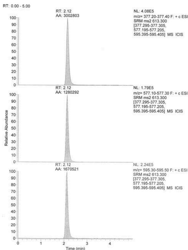
Figure 1. Chromatogram of a grease sample containing  $0.4 \text{ mg kg}^{-1}$  of lasalocid.
