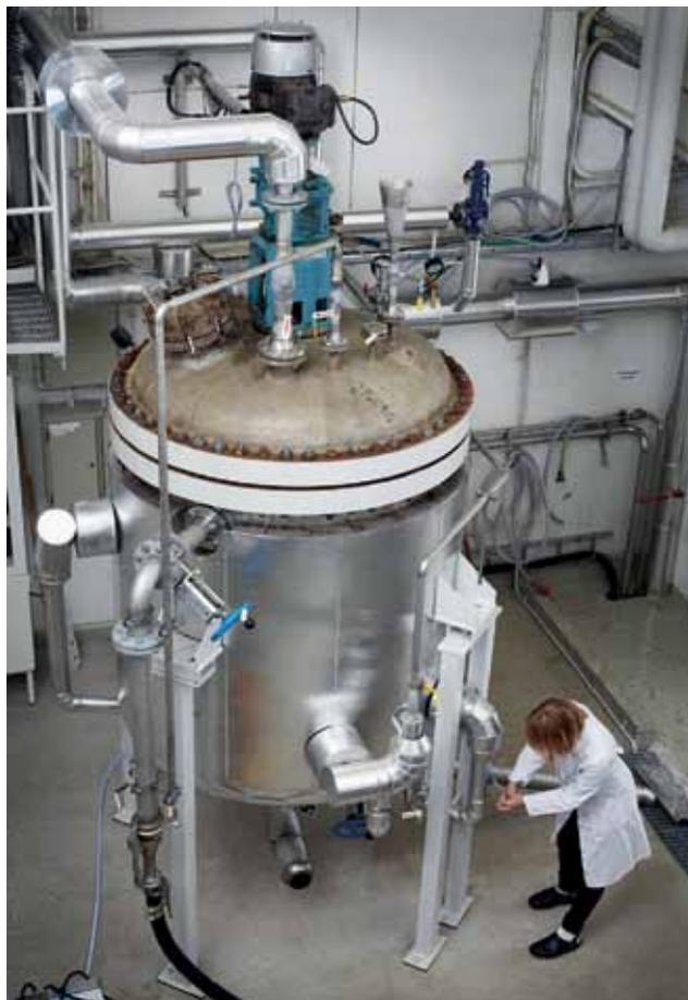
The Innventia pilot plant in Stockholm produces 100 kg/d of nanofibrillated cellulose
