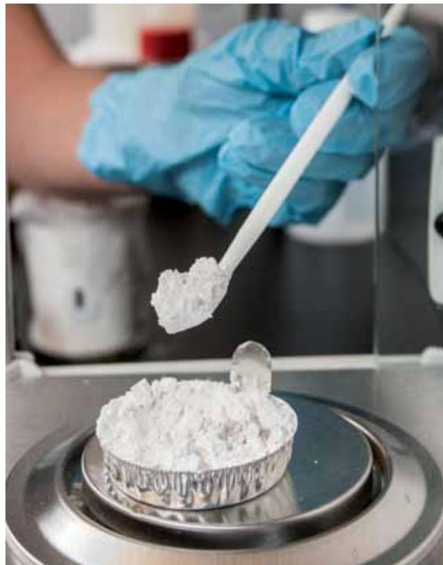
Nanocellulose crystals shown here can produce composite materials stronger than steel
