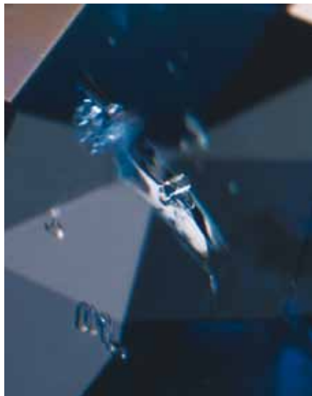
Figure 7: Mineral inclusions of the spinels heated at relatively lower temperatures also revealed evidence of this treatment. Shown here are inclusions of apatite with thermally induced stress fractures. (Photomicrograph: Christopher P. Smith, 65x)
