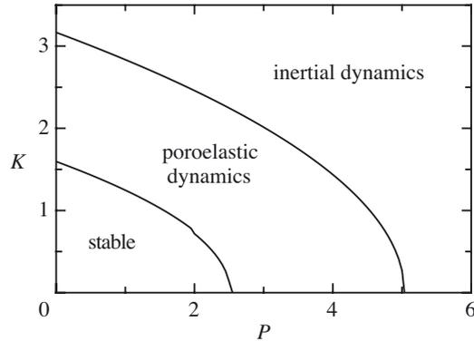
Figure 12. For the case of an applied compression  $P$  and axial twisting moment  $K$ , we show the three short-time regimes (stable, poroelastic, and inertial) as in figure 4.  $E = \delta = 1$ .
