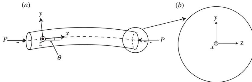
Figure 1. Schematic of (a) a bent rod, where  $\theta(x)$  is the angle between the deformed and undeformed tangent vector and  $x$ ,  $y$  and  $z$  are body-fixed coordinates in the reference frame of the rod; (b) the circular cross-section.
