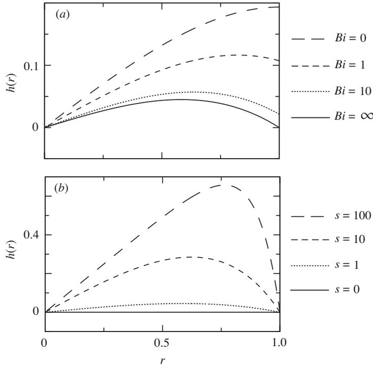
Figure 5. The radial variation of the fluid pressure at the onset of buckling,  $h(r)$ , for (a) growth rate  $s = 1$  and various values of the surface permeability parameter  $Bi$  (larger  $Bi$  corresponds to a more permeable surface) and (b)  $Bi = \infty$  and various  $s$ .
