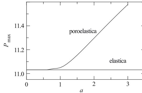
Figure 10. Maximum compressive load,  $P_{\max}$ , for displacement-controlled buckling, where the displacement field is given by  $\Delta(t) \approx 0.1[1 + \tanh at]$ .  $Bi = 0.1$ ,  $\delta = 1$ ,  $dt = 0.01$ ,  $dx = 0.01$ .
