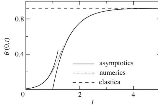
Figure 7.  $\theta(0, t)$  for  $P = 11$ ,  $\delta = 1$ ,  $Bi = 0.1$ ,  $dx = 0.01$ ,  $dt = 0.001$  and  $\theta(x, 0) = \theta(x, dt) = 0.01 \cos \pi x$ . The short-time asymptotic is for a growth rate  $s(P)$  found from equation (4.9). The long-time asymptotic is of the form  $Ae^{-\psi t} + \theta_0$ , where  $\psi$  is the rate of decay to the equilibrium angle  $\theta_0$  and  $A$  is a fitting parameter.
