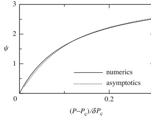
Figure 6. As the solution approaches the equilibrium shape, the difference between the current and equilibrium shape decays exponentially with a rate  $\psi$ , which is plotted against the applied compression.  $\delta = 1$ ,  $Bi = 0.1$ ,  $dx = 0.01$ ,  $dt = 0.01$ . The numerical computation is begun with  $\theta = 0.9\theta_0$ .
