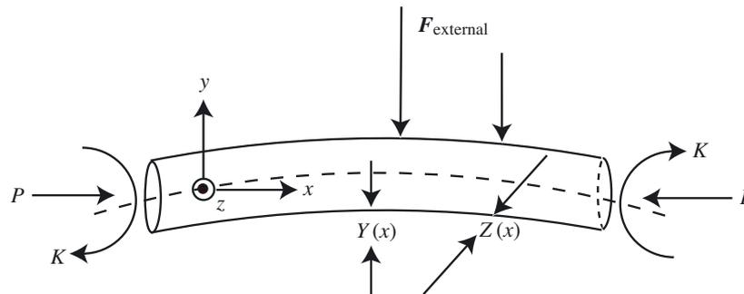
Figure 11. Schematic of a rod buckling under an applied twist and compression in an external medium.  $Y(x, t)$  and  $Z(x, t)$  are the displacements of the centreline in the  $y$ - and  $z$ -directions respectively. The dotted line denotes the axis of symmetry.
