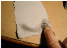
Step 3: Sharpen around the entire end of the blade and the one-inch cutting edge. Keep the angle very flat, as shown. Sharpen both sides of the blade, turning often to keep the edges even—if you prefer a single bevel, sharpen the side of the blade that will face up when you use it (this will vary depending on whether you are right- or left-handed).
