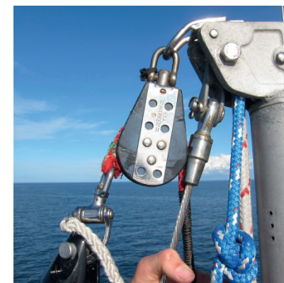
▲ Above: the Colligo continuous-line furling gear for a Code 0 on Schell's Arcturus; note its position forward of the headstay. Left: the masthead spin halyard is clipped to the upper swivel on the Colligo Code 0 furling gear, though do not let the spin halyard and block touch the headstay as here
