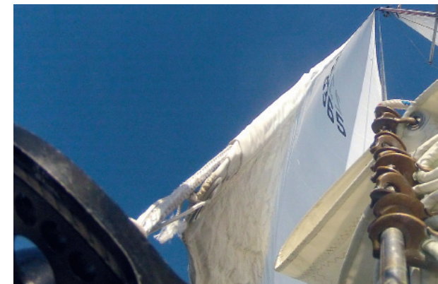
▲ Above: the Colligo continuous-line furling gear for a Code 0 on Schell's Arcturus; note its position forward of the headstay. Left: the masthead spin halyard is clipped to the upper swivel on the Colligo Code 0 furling gear, though do not let the spin halyard and block touch the headstay as here
