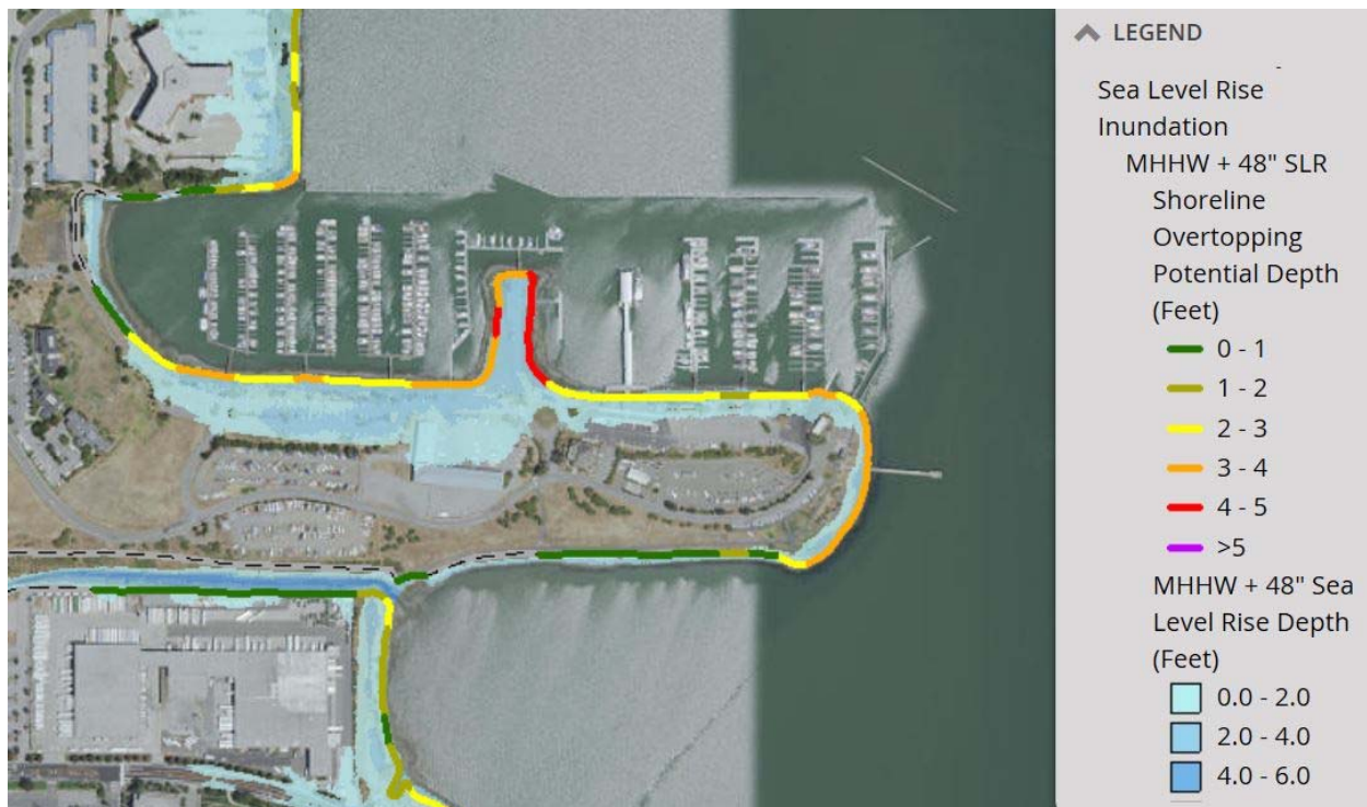
Figure 1 - Oyster Point Landfill with 48" sea level rise (image from the SMC Vulnerability Assessment ARCGIS Website)
