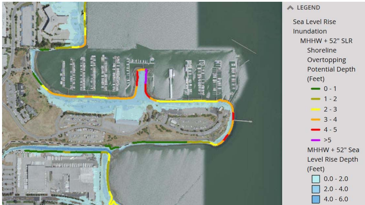
Figure 3 - Oyster Point Landfill with 52" sea level rise (image from the SMC Vulnerability Assessment ARCGIS Website)
