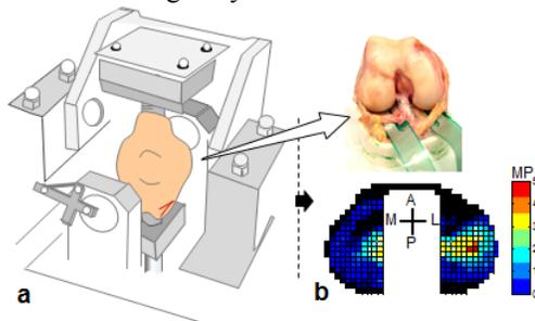
**Figure 1** (a) Experimental setup of the dynamic knee joint simulator. (b) Contact stresses on the tibial plateaus measured by Tekscan sensor.
