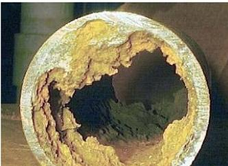
Cut-away section of pipe showing internal corrosion. (Example shown is not from EPA buildings.)
