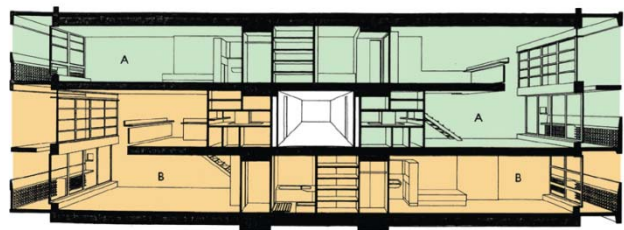
Fig. 5: Unité d'Habitation, cross-section showing units with 'double orientation' and brises-soleil on the east and west.
