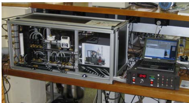
Figure 2. FTIR analyser installed in the Cape Grim main laboratory.
