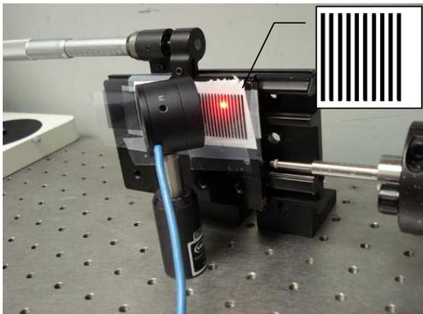
Fig.3 Ronchi Rulings on a linear stage, LVDT was attached to the right edge to measure the displacement.
