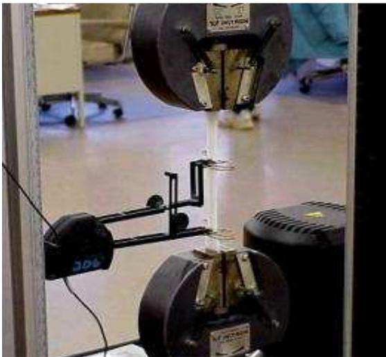
Fig.1 A mechanical extensometer clamped on a stretched material specimen.
