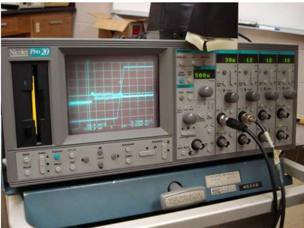
Fig.8 Data acquisition system with 2 channels on. Channel one is for LVDT. Channel two is for photo detector.
