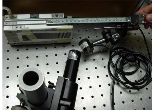
Fig.4 The manual linear stage is replaced with an air actuated linear stage to carry out the high pressure test.
