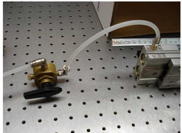
Fig.5 The pipe used to actuate the linear stage with high compressed air. On the left is a switch used to deflate the stage and move it back to original position.
