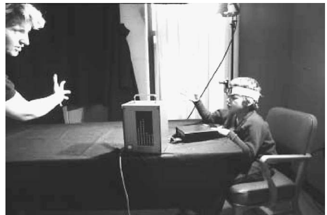
Fig. 10. The optacon device is used both for reading printed text and for viewing an environment, both through its 6 \times 24 pin tactile display. As noted in the original caption of this figure, reproduced from Bach-y-Rita et al. (Bach-y-Rita and Kercel, 2003), the child is able to mimic the hand posture of the teacher using feedback acquired via the device.
