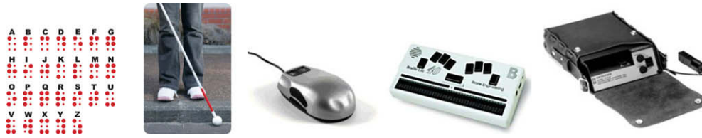
Fig. 9. Pictorial collage of sensory aid devices. Left to right: The Braille alphabet, the long white cane, the VTPlayer mouse (a mouse with integrated tactile pin array), an electronic Braille reader, and the Optacon.
