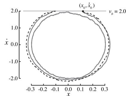
Fig. 7: Two phase-space trajectories of the Langevin system, near the critical speed for stick-slip motion, integrated from  $(x_0, v_0)$  until first passage. Dashed line: fundamental mode (mean period  $\tau$ ). Solid line: A double orbit ( $\tau' \approx 2\tau$ ).  $D = 3$ ,  $v_b = 2$ ,  $\omega_0 = 1$ ,  $\zeta = 0.02$ .
