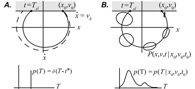
Fig. 3: (A) Periodic phase-space orbit produced by a simple deterministic friction law. (B) Dynamics in a stochastic friction model with a distribution  $p(T)$  of periods. The state follows a transition probability density  $P(x, v, t | x_0, v_0, t_0)$ . The ellipsoids represent level sets (isolines) of this density at successive times.
