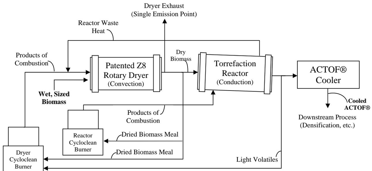
**Fig: ECP's Torrefaction Process**
