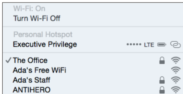
Figure 6: Instant Hotspot puts an iOS device into your Wi-Fi menu in OS X.
