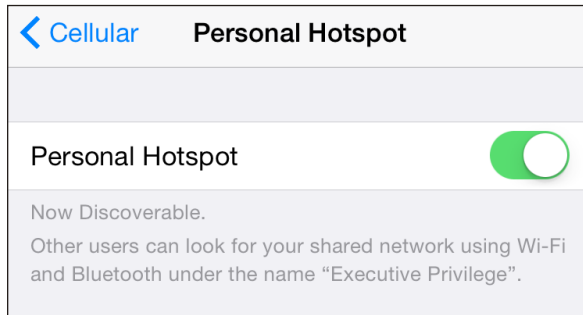
Figure 5: The Personal Hotspot view lets you turn access on or off as well as set a Wi-Fi password.
