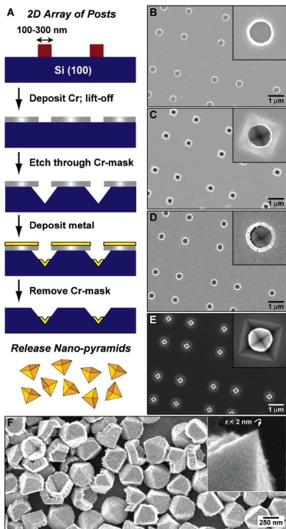
**FIGURE 6.** (A) Scheme depicting the fabrication of the free-standing metallic pyramids, (B) Cr mask of 250-nm holes, (C) etched Si(100) pyramidal pits undercutting the Cr mask in panel B, (D) 50-nm film of Ni deposited on the structures in panel C, (E) Ni pyramids situated in the centers of the etched Si pits (the insets are 500 nm  $\times$  500 nm), and (F) released metallic pyramids (inset—tip of a Au/Ni/Au pyramid with  $r < 2$  nm). Adapted from ref 20.
