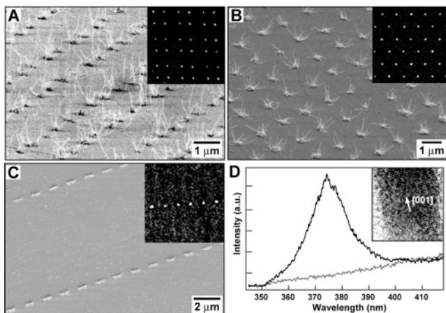
**FIGURE 3.** Arrays of ZnO nanowires grown from Au dots: (A) square lattice; (B) hexagonal lattice; (C) 1D arrays; (D) photoluminescence from ZnO nanowires patterned in a square lattice (inset—HRTEM image of a ZnO nanowire). Adapted from ref 18.
