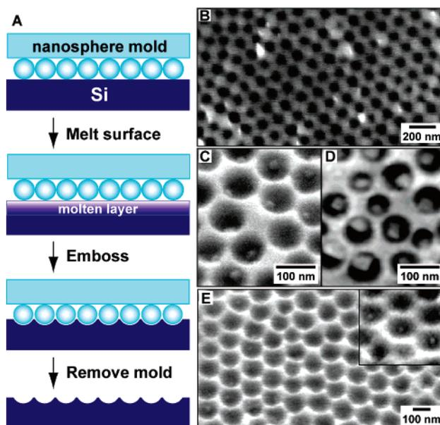
**FIGURE 1.** (A) Scheme for generating nanowells, (B) nanowells in Si, (C) NaCl crystals from 1 M salt solution, (D) NaCl crystals from 5 M salt solution, and (E) CdS nanocrystals in nanowells (inset—zoom of CdS nanocrystals). Adapted from ref 17.
