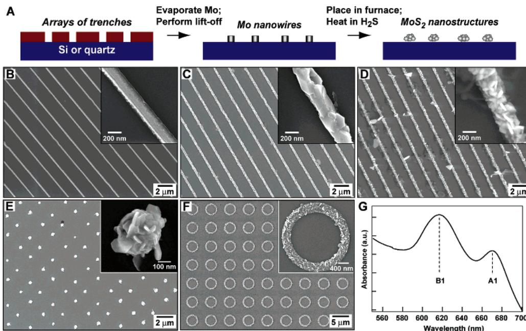
**FIGURE 4.** (A) Scheme for patterning MoS<sub>2</sub> nanostructures, (B) lines of Mo, (C) MoS<sub>2</sub> lines converted from panel B after reacting with H<sub>2</sub>S gas, (D) MoS<sub>2</sub> lines converted from panel B with crystals oriented perpendicular to the surface, (E) MoS<sub>2</sub> dots, (F) rings of MoS<sub>2</sub> nanostructures, and (G) UV–visible absorption spectroscopy of a MoS<sub>2</sub> nanostructured film. Adapted from ref 19.
