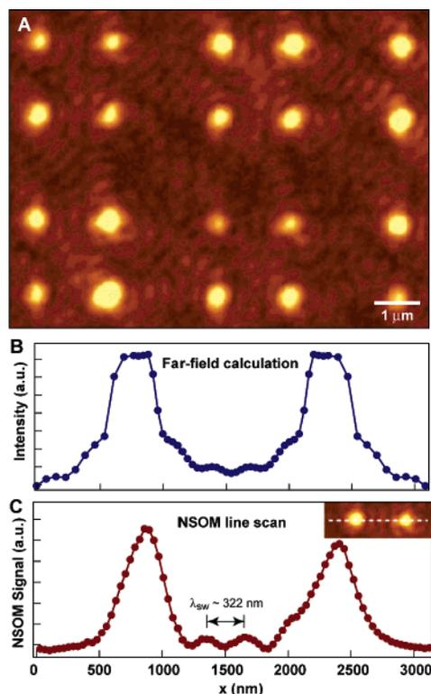
**FIGURE 8.** (A) NSOM optical image of holes in a 100-nm Au film on glass, (B) calculated far-field intensity of four holes, and (C) cross-section of two neighboring holes from panel A. Adapted from ref 31.
