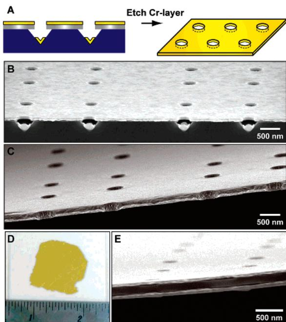
**FIGURE 7.** (A) Scheme to release free-standing film of large-area nanohole arrays, (B) nanohole film attached to Si with pyramids beneath the holes, (C) portion of a free-standing 100-nm Au film perforated with 250-nm holes, (D) optical micrograph of  $\sim 1$  in.<sup>2</sup> film on a glass, and (E) portion of a free-standing Au/SiO<sub>2</sub>/Au film. Adapted from ref 31.
