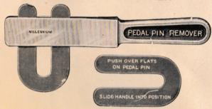
This handy tool enables pedal pins to be removed without dismantling The ordinary type of spanner, even if thin enough on the jaws to go in the space provided, has not sufficient strength to withstand the strain.
