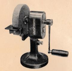
The Driving Mechanism is substantial and readily gives the necessary high speed for satisfactory grinding, the whole being enclosed in a grease-retaining dust-proof cover.
