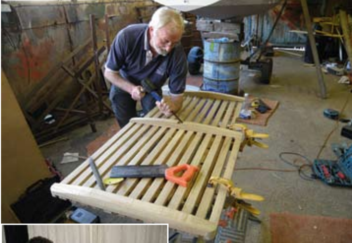
ABOVE Dick works on a removable teak grating for the cockpit floor
