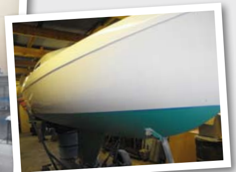
...followed by three coats of Perfection Topcoat and FLAG cruising antifouling
