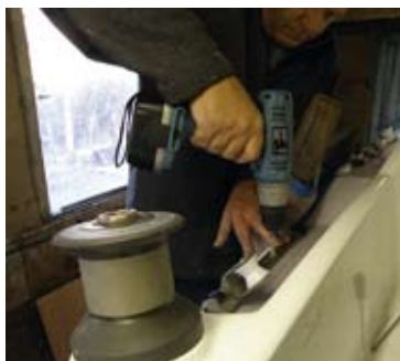
New winches and genoa tracks could be bolted on once the paint had cured
