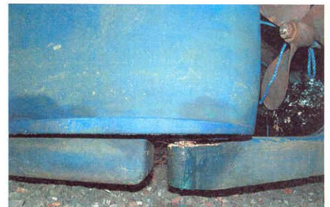
Main: Despite a general discolouration – more likely caused by the boat being dried out in some very muddy harbours – there is no sign of animal growth or weed and only the thinnest smear of sliminess. The thinness of the antifouling along the leading edge of the keel was caused by abrasion when the crane's lifting strops were pulled into position Below left/right: Apart from minor barnacle growth near the rudder stock, the rudder area was pretty clean
