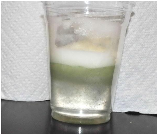
Figure 6. Coagulated microalgae (Sample A) immediately following EC treatment
