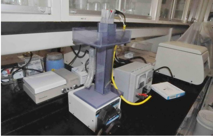
Figure 1. The bench-top electrocoagulation set-up, with capacity of 1 liter per minute, continuous flow.
