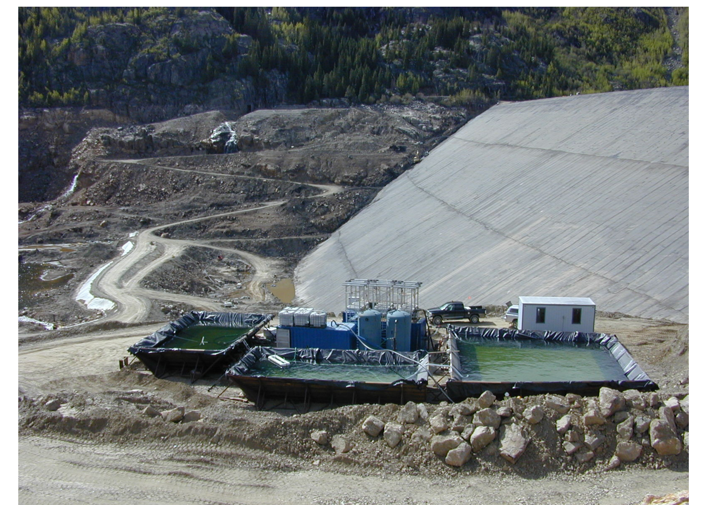
Figure 3: The EC system was set up to treat water that had been used in the resurfacing of a dam. The water was recycled for reuse.
