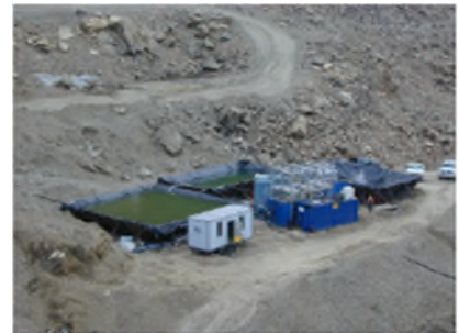
Figure 1. The above picture was taken of an electrocoagulation system that was being used in a silver mining project in Colorado.
