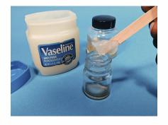
approx. three half-full eyedroppers of mineral spirits. The petroleum jelly is thick, so instead of trying to shake the mix by hand or hand string, I used a hobby electric paint mixer to throughly blend and mix the components
