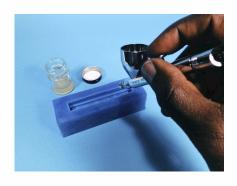
an air pressure to approx. 15 psi. if using a gravity feed airbrush. For bottom-feed airbrushes, dial in 20 psi.
