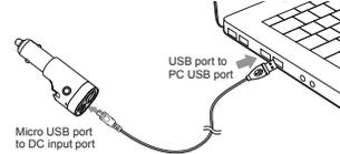
**USING AN EXTERNAL USB POWER SOURCE:** Use the provided USB cable to connect the car charger micro USB port and the USB power supply USB port. When charging the green charging indicator will be flashing and the blue working indicator will light up. When the battery is full, the indicator will stop flashing and all green energy indicators will light up.
