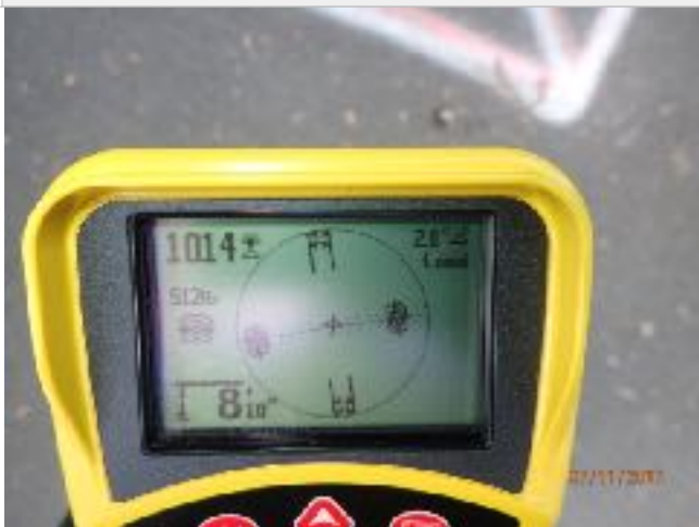
Approximate depth and location of sewer tap. Surface view
