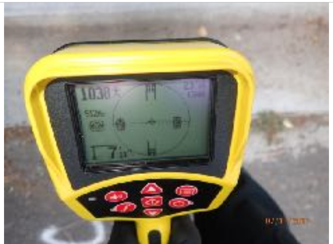
Offset ~7' - 8' deep at the at the storm curb
