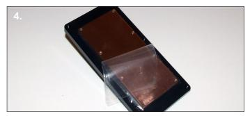
**4.** Remove the protective tape from the waterblock's copper base ready for installation.
