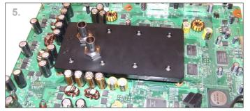
**5**. Place the waterblock over the CPU and GPU making sure the holes on the board line up with the edges of the waterblock. With one hand on the waterblock carefully turn the board upside down.
