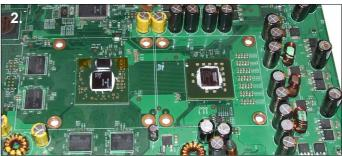
**2.** Clean the CPU and GPU to remove any residue left from the thermal pads.
