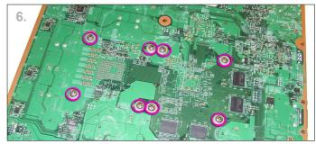
**6**. Finally use the 8 screws and 8 washers to attach the waterblock. It is best to start by screwing in all 8 screws loosely. When you are happy with the position of the block gradually tighten each of the screws. It is important not to overtighten the screws as this could damage the CPU or GPU.
