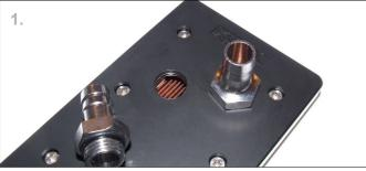
**1**. Screw the barbs into the G1/4" ports using an adjustable spanner. Make sure the o-rings are fully compressed.
