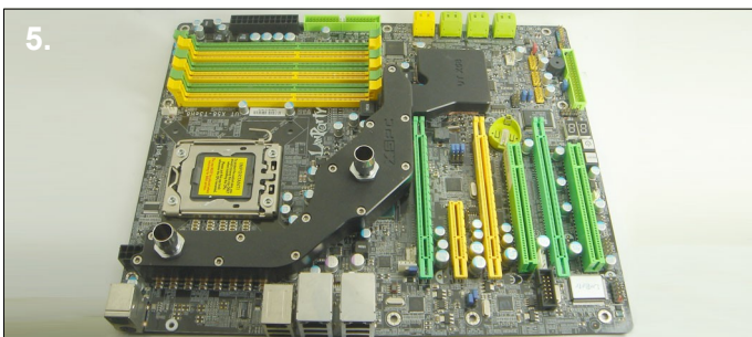
5. Carefully place the waterblock onto the motherboard making sure the screw holes line up and the thermal pads stay in place
