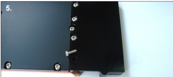
5. Use the four 8mm screws to attach the aluminium bridge the the waterblock.
