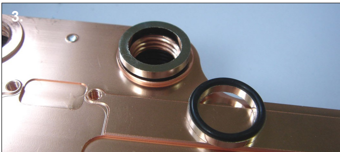
3. If you are using G1/4" barbs/fittings with a long thread you will need to use the supplied rings to avoid blocking the flow.
