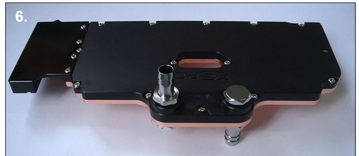
6. The block is now ready to be connected to the other watercooling components for leak testing.
