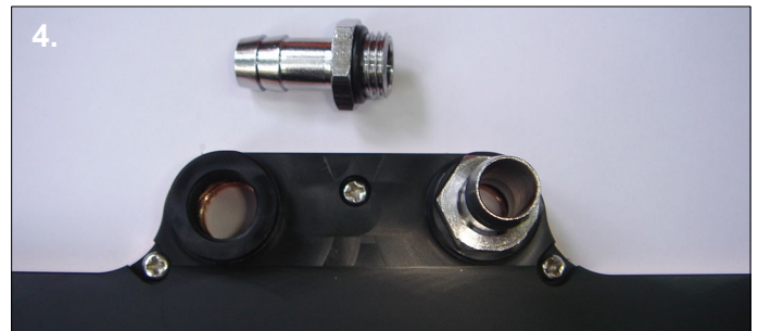
4. Attach the barbs to your chosen ports using an adjustable spanner. Make sure the o-rings are fully compressed.
