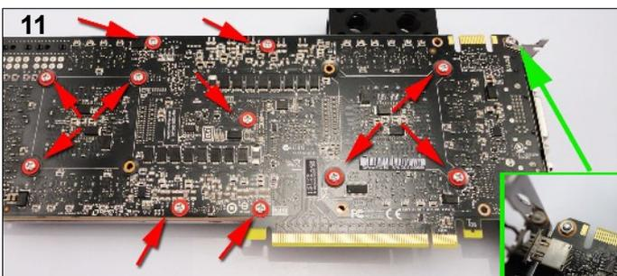
**11.** Place the waterblock on the card to line up the screw holes and then flip it over, making sure the thermal pads stay in place. Now carefully attach the block to the card using twelve M3 screws and washers. The screw marked in green requires an M3 nut attaching on the other side of the card.
