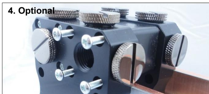
**4. Optional** If you are using cards in SLI you can use the optional SLI flow connector to bridge the two cards. This should be done after step 12.
