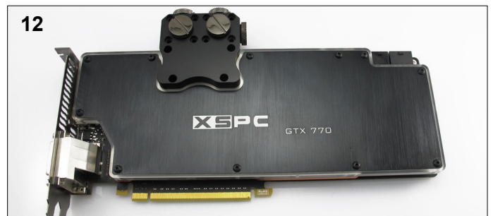
12. Do not over tighten the screws as this may bend the card and cause permanent damage. The card is now ready for use. When you first boot it is advisable to use software to check the core temperature. If the temperature is high you will need to remount the block.
