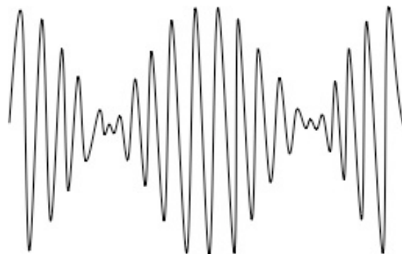
Figure.2 - Resulting beats waveform of two tones with slight frequency difference (after Rasch and Plomp, 1999).
