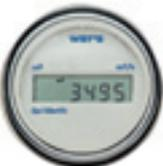
Electronic register showing rate of flow and accumulated volume. The register has LCD with 6 digits. The register has interchangeable presentation (every 30 seconds) between the rate of flow and volume. Mounted inside stainless steel vacuumed encapsulated cup with glass lens, hermetically sealed IP 68. Can be installed on any Arad meter and hydrometer.
