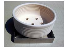
You can sit your pot melt pot right on the stainless steel for support. Just be sure to calculate the amount of glass you use. You can also put it up on supports to have the glass drop farther for a different look. Of course these forms still need 1/8" thick fiber paper before firing!
