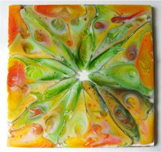
1/ Once the melt has been removed from the kiln, with either diamond hand pads or a grinder smooth the outer edge making sure all the fiber paper is removed. A 120 grit or higher will do.
