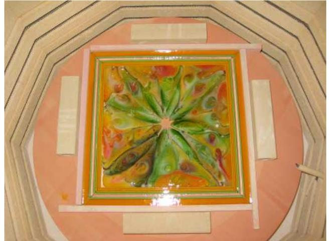
Please note; some glass is very inconsistent in thickness which will cause the lines to curve or wiggle ever so slightly. If you used this type of glass in your strip cut border I recommend firing face down then flip and fire polish.
