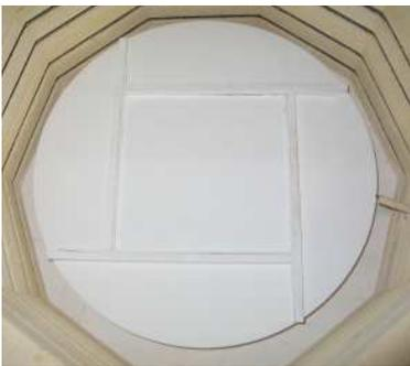
Place a 12" square piece of shelf paper on a newly washed kiln shelf and place a 10" square of clear thin glass on top of the shelf paper. Add barriers or glass dams around the perimeter lined with 1/8" fiber paper. Cut each fiber paper strip 10-1/2" long and 5/8" wide. It can measure anywhere between 5/8" and 1" wide but must be at least 1/2" longer than the glass so the dams can be pushed up against the fiber paper.
