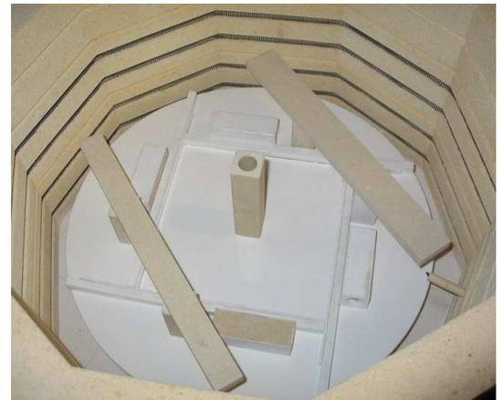
Position 4 kiln posts on the outside of the barrier and balance two horizontal supports on top. The Annular ring pot will sit on these. If necessary place additional kiln posts or equivalent against the glass dams to prevent the barriers from moving. Place a tall kiln post or something equivalent in the exact center of the glass. This is to help center the pot and will be removed.
