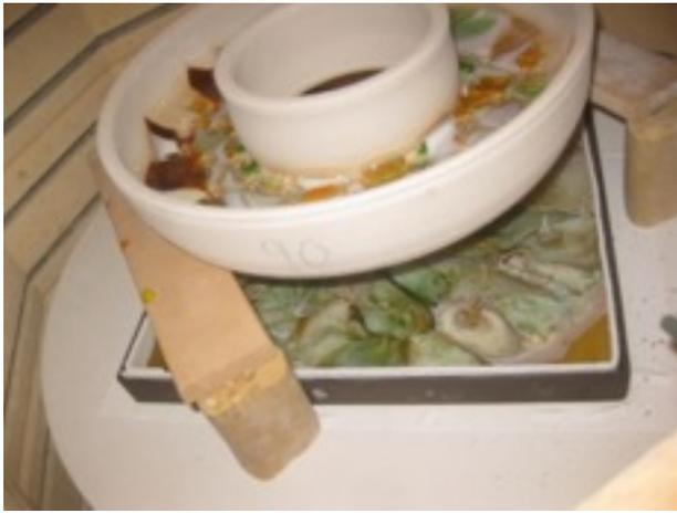
Here is a photo of an Annular Pot Melt Ring that has been fired over a square Stainless Steel form. As long as the holes are inside the fiber paper you are good for any shape form.
