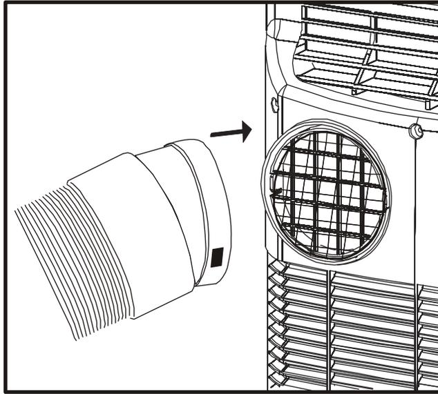
7. Align the slots on the duct connector to the tabs and snap into the back of the unit.
