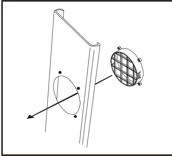
1. Insert the round grated adapter through the back grooved side of the window kit plate with hole.
