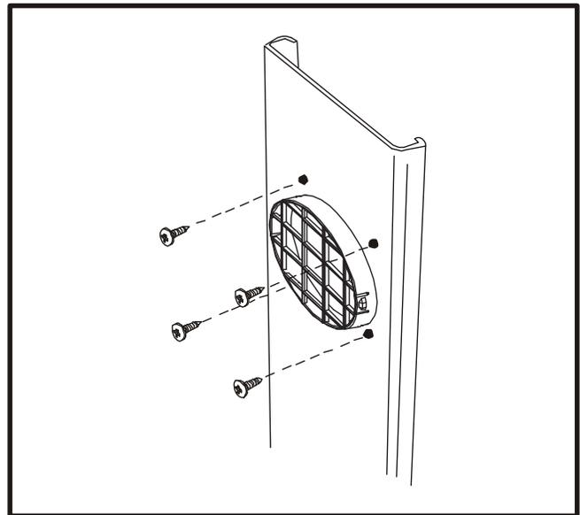
2. Secure the grated adapter by fastening the screws from flat side of the window kit plate to the holes on the grated adapter.
