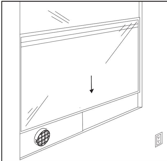
4. Lower the window to secure the window kit in place. You may need to use duct tape to better secure the window kit.
