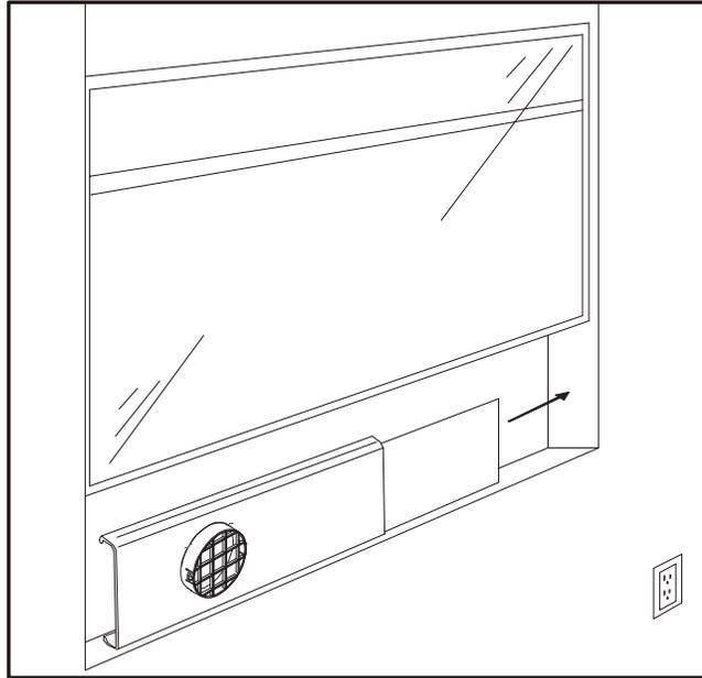
3. Open your window and place the window kit with grooved side facing outward on the window sill. Then, slide the window kit plate to fit the width of the window. You can use screws to secure the window kit plate from sliding.
