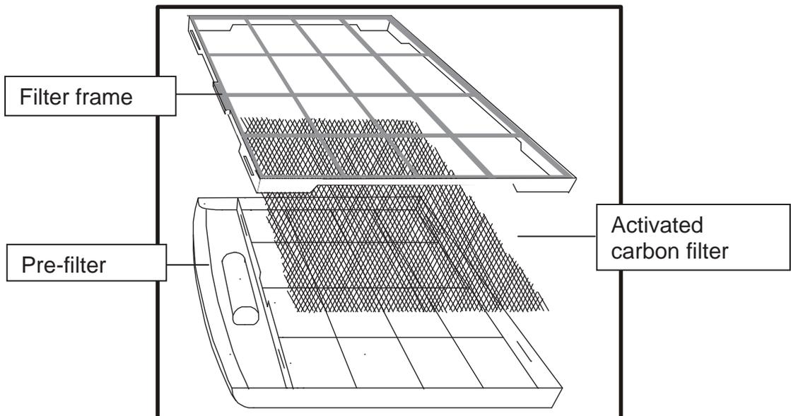
2. Separate the filter frame from the pre-filter.
