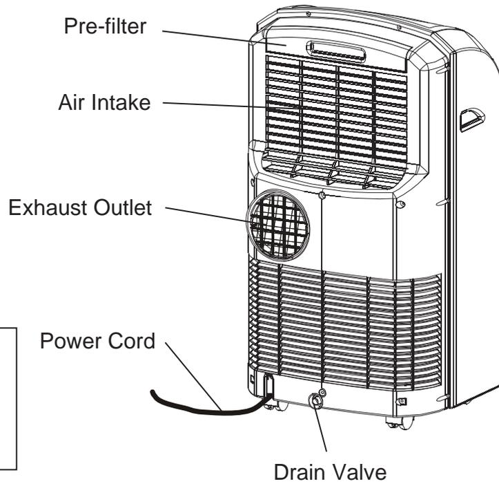
**CAUTION:** Make sure the drain plug is firmly installed before using the unit. This will prevent leaking.
