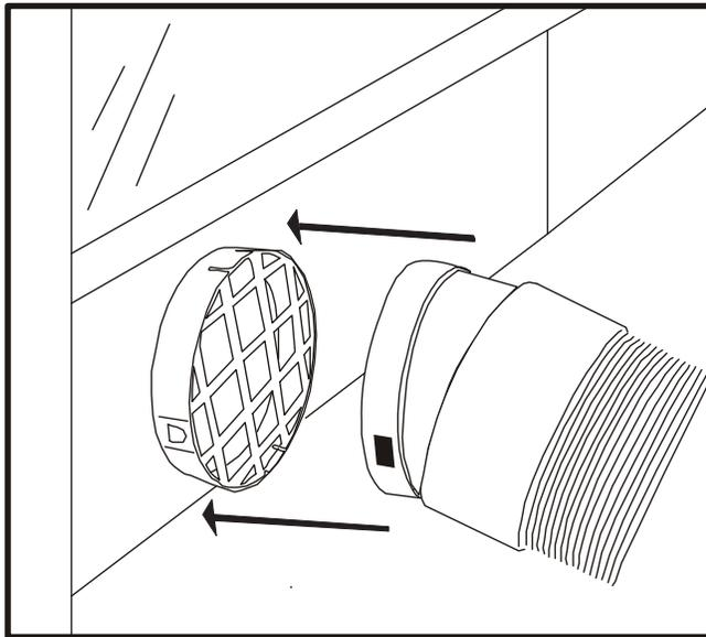
8. Align the slots on the duct connector to the tabs on the grated adapter and snap in place.
